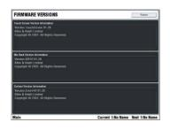
**Firmware page** Lets you check the current system firmware versions and load in new firmware using a USB key.
